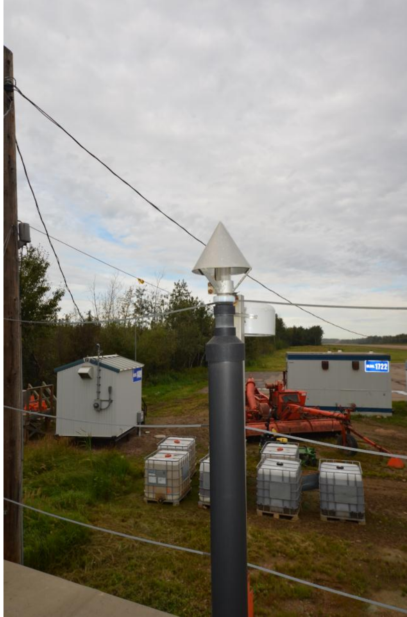
Figure 4.6 – Outdoor Sample Inlet
