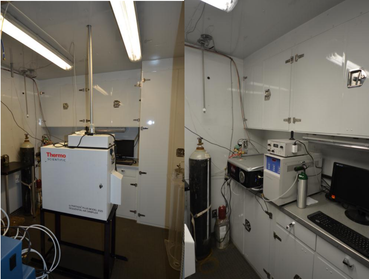
Figure 4.5 – Sequential Dichotomous sampler & VOC Technologies, Pneumatically Focused Gas Chromatograph
