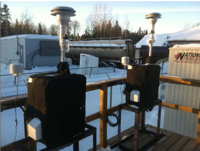
Figure 4.3 – PM2.5 and PM 10 samplers
