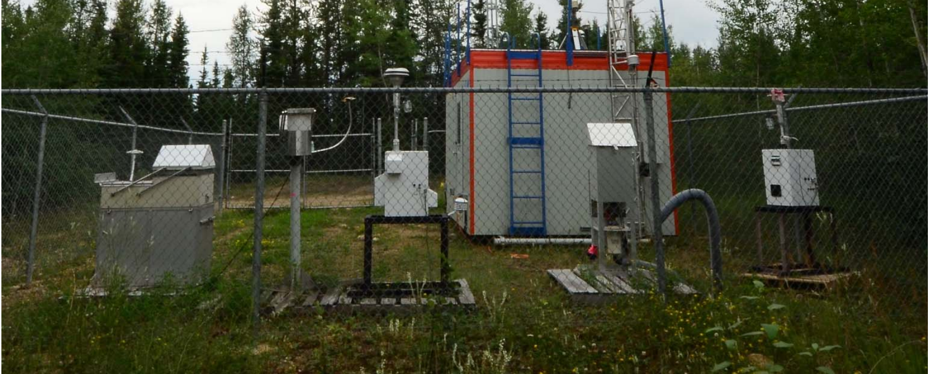
Figure 4.8 – Samplers, left to right: EC organic precip, EC inorganic precip, EC PM2.5, High volume PUF, PM10
