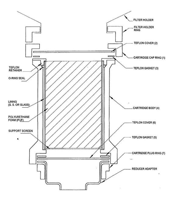
FIGURE 2 POLYURETHANE FOAM ( PUF ) CARTRIDGE ASSEMBLY
