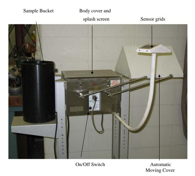
Figure 1.1 Precipitation Collector
