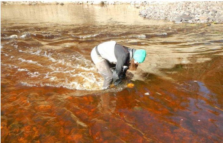
Figure 1. Crew member collecting a water sample from a riffle (facing upstream, with a bottle lowered to approximately half of the stream's depth).
