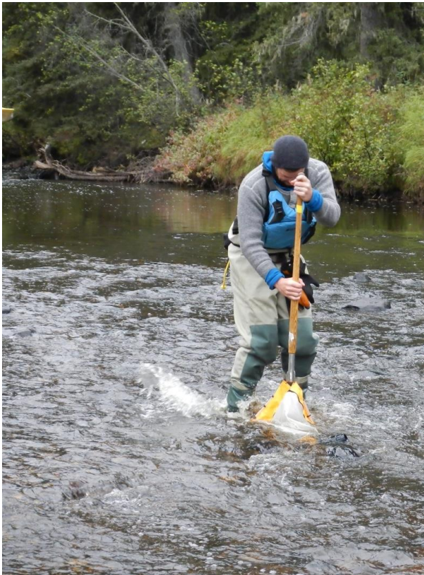
Figure 1. Crew member performing the CABIN 3-minute travelling kick to collect benthic invertebrates from a riffle.
