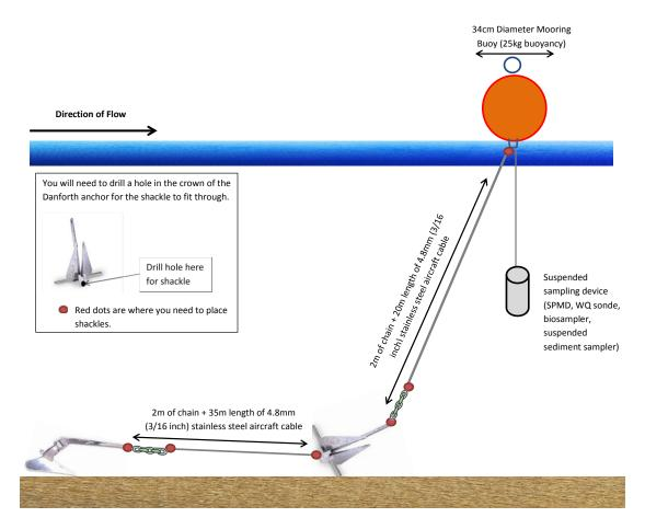
Figure 1. Open-water array design.
