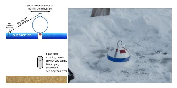
Figure 2. Suspended under-ice design.
