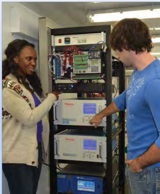
HEMP Program Manager, Abena Twumasi-Smith and Technician, Zach Eastman, calibrate the odour analyzing instruments in the HEMP Portable air monitoring station.
